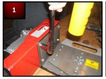
Remove four bolts that secure motor housing to base plate.
