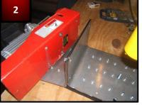
Remove motor housing from base plate assembly and set aside.
