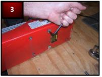
Remove two allen bolts that secure motor to motor housing.
