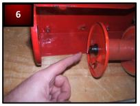
While motor is clear from assembly grease spool liberally.
