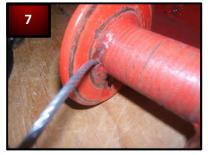
Feed cable into spool as shown.
