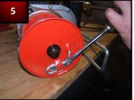
Remove key chuck retainer with a screwdriver and remove cable.
