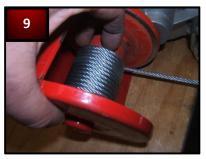
Feed end of cable into spool retainer clip as shown. Pull cable length for secure fit.
